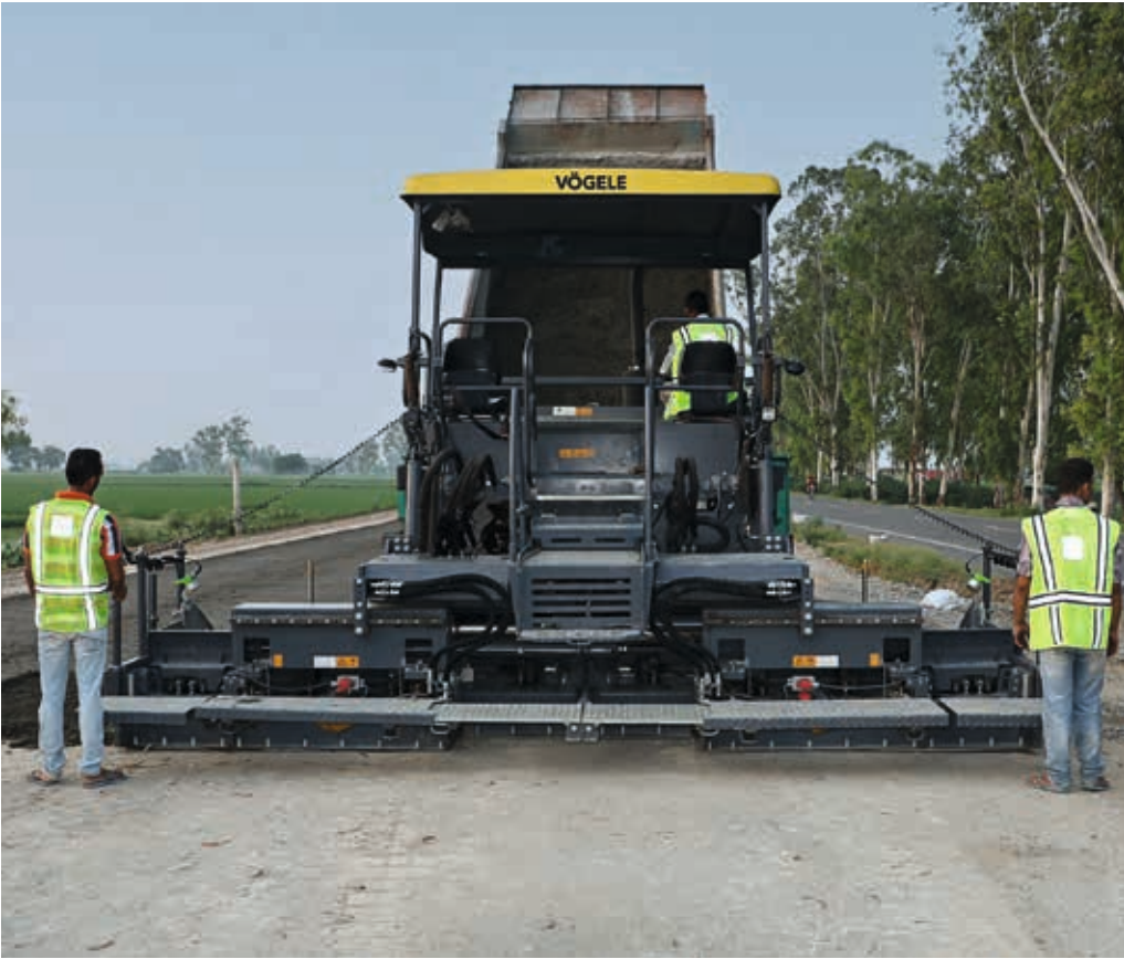
> Left: Combined with the cutting-edge AB 480 TV Extending Screed, the SUPER 1400i is capable of building high-quality pavements in varying widths up to 7.5 m through the addition of bolt-on extensions. Bottom: The large and sturdy material hopper of the SUPER 1400i holds 13 t. Thanks to the low and wide hopper sides, feeding the paver with mix is a fast and easy process.
