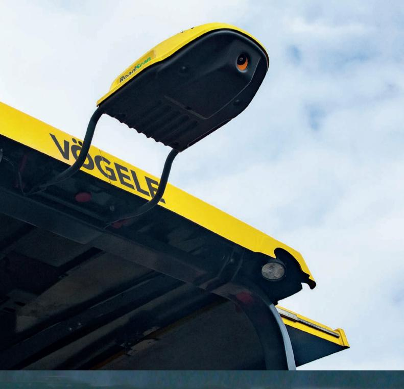
RoadScan, VÖGELE's temperature documentation system, optimally meets the requirements specified by authorities inviting tenders in terms of temperature range, measured width, measurement density and analysis.
