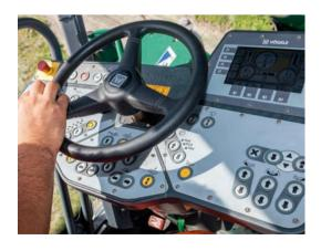
Intuitively designed paver operator's ErgoPlus 3 console: the SUPER 1803-3i wheeled paver can be controlled easily and precisely using the steering wheel.
