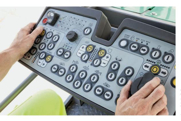
Leading technology that's easy to use: the SUPER pavers and VÖGELE screeds are operated with the intuitive ErgoBasic operating concept.
