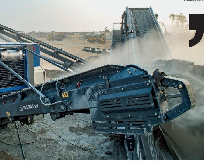
A team player: the screens operate particularly efficiently when linked with crushers of the EVO series that are configured in size and output to the MS EVO screens.
