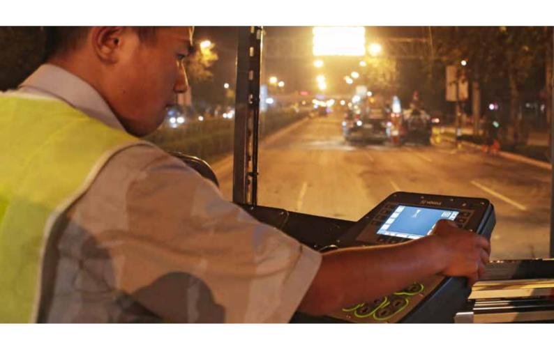
The SprayJet module is operated entirely via the touch screen integrated into the spray module.
