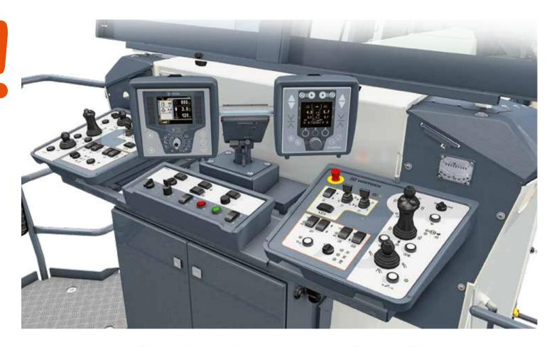
The very clear arrangement of the controls and the robust operating display simplify operation of the W 215.
