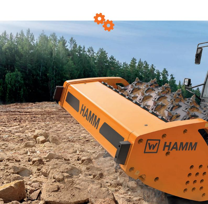
Breaking and compacting rock in a single pass - this is just what HAMM developed the 3625 HT VC compactor with crusher drum for. The key component of the 25t machine is a 2.22m-wide VC drum (VC = vibration crusher) with 150 picks. They break up the hard rock material with extremely high point loads while it is compacted by the vibrating drum.
