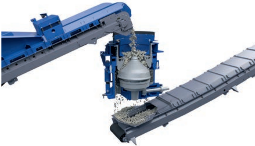
Crushing mechanism of cone crusher
