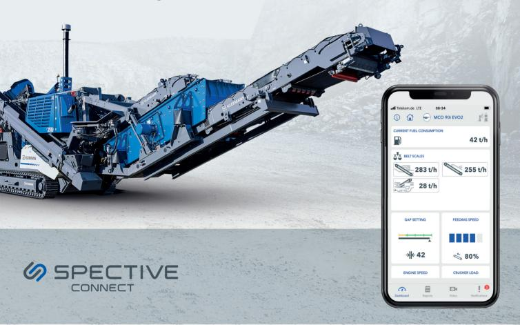
The crushing capacity of a crushing plant can now be conveniently determined via integrated belt scales (optional) on the discharge conveyors. Using SPECTIVE CONNECT, this data can now be displayed not only on the SPECTIVE touch display but also on the smartphone.
