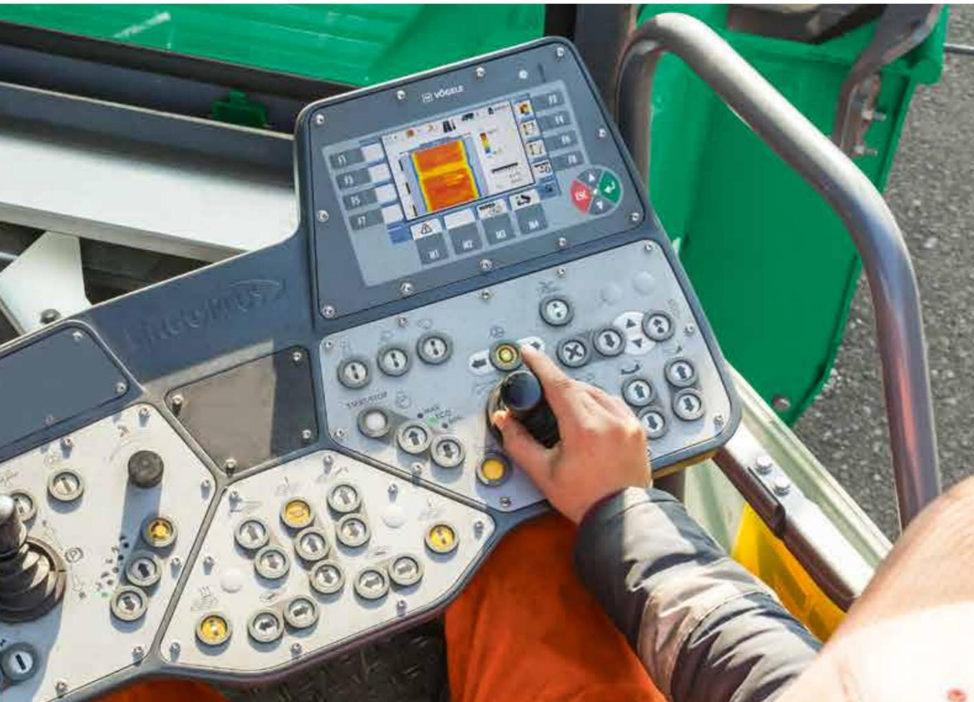
The paver operator is linked to the job site module via the ErgoPlus 3 display. For example, he can access current information on the job site and the progress of the project at any time. Thanks to clearly arranged and easily comprehensible diagrams, he can immediately recognize a deviation of the actual situation from the plan.
