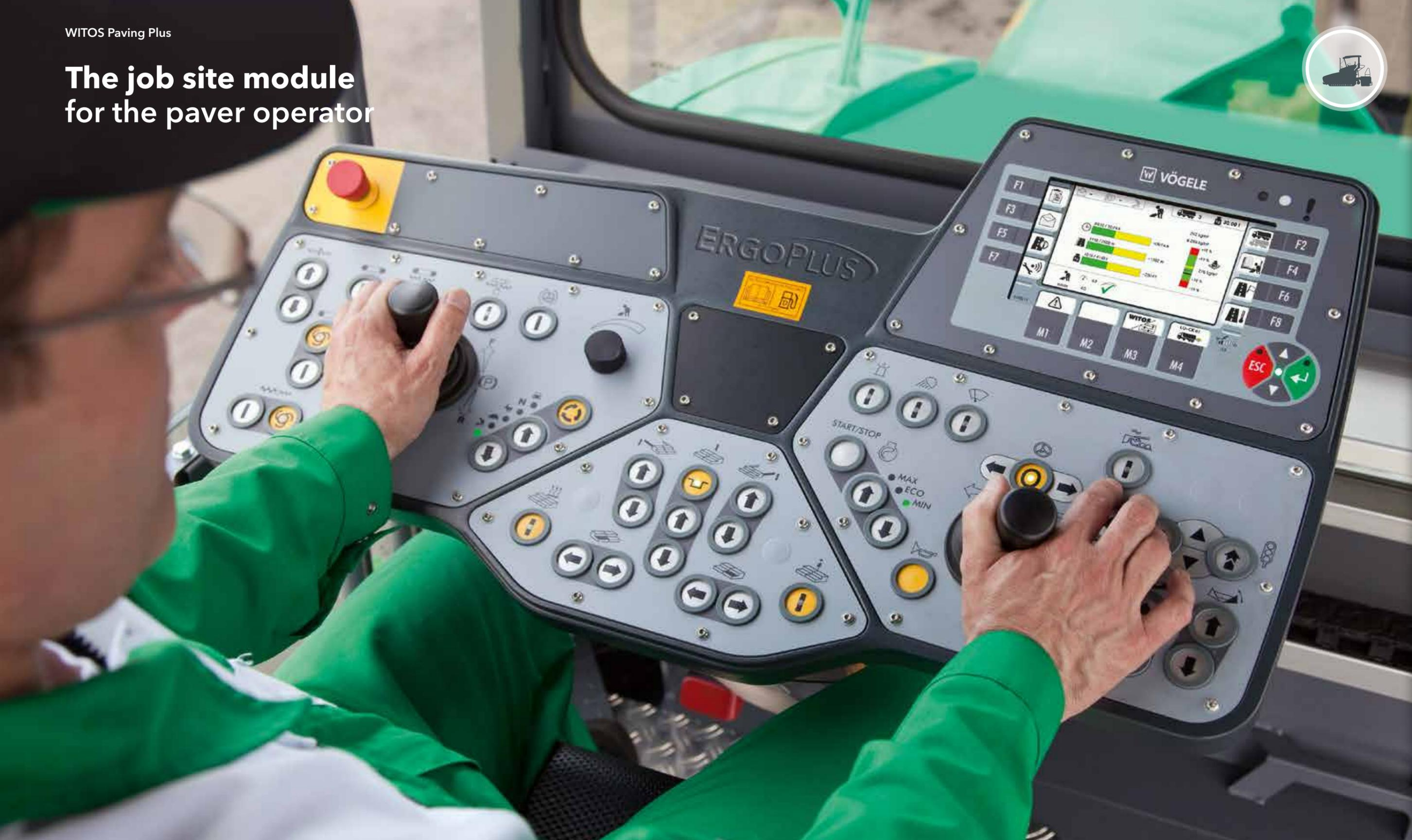
**The job site module** is an integral part of the VÖGELE ErgoPlus 3 paver operating system and offers the paver operator a unique tool for control and process optimization.
