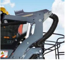
NO DISMANTLING: the exhaust air pipe is folded down with the roof for the purposes of transport.\*
