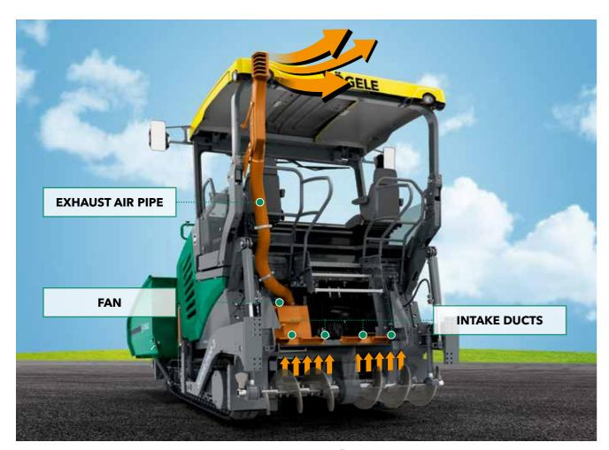
Please note: the design of the ventilation systems supplied by VÖGELE differs depending on the series in question. The pictures show the system for the SUPER 1900-3(i) and SUPER 2100-3(i) pavers by way of example.
