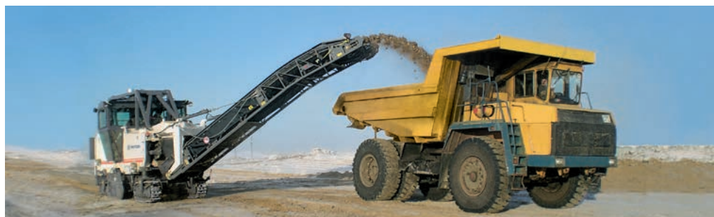
Surface Miners cut, crush and load the material in a single operation with just one machine
