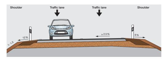
When performing soil improvement operations at subgrade level, the edge design of embankment structures may require excess profiling due to the production methods and equipment used.
