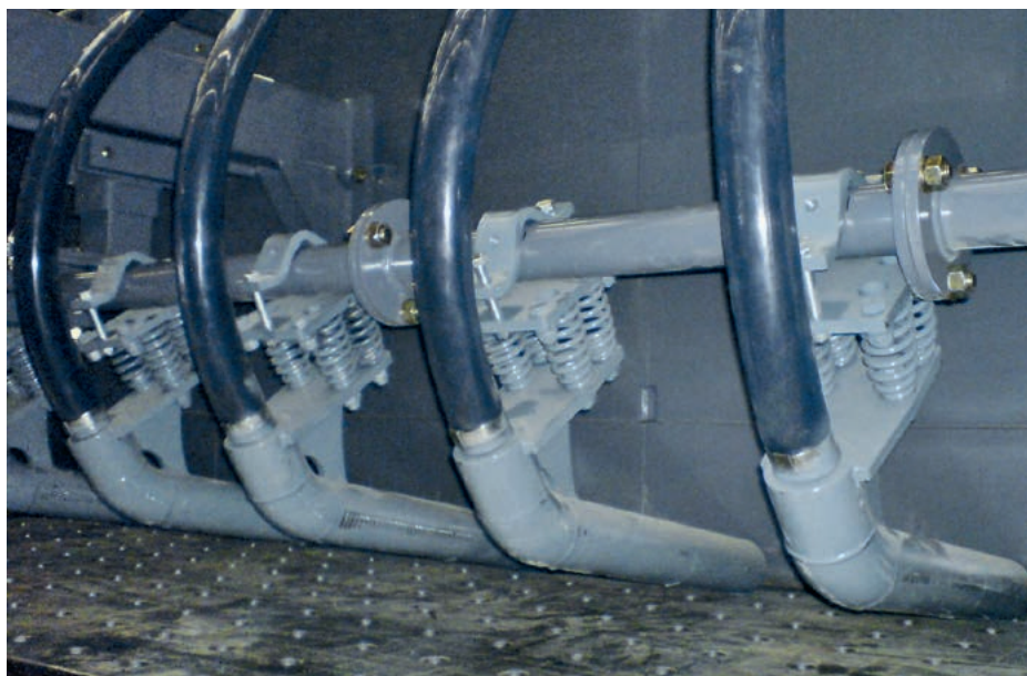
The vibrators are arranged at regular intervals
