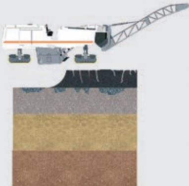
Mill off all asphalt
