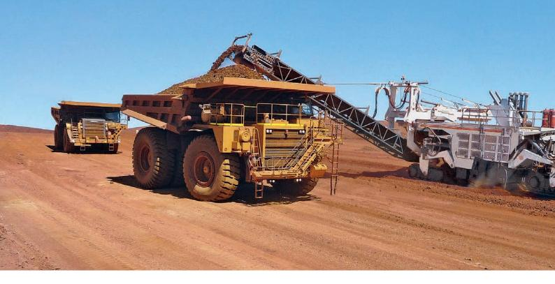
One of the WIRTGEN surface miners' most important features is their ability to load the cut material directly onto trucks, like the 4200 SM shown here. The belt can be pivoted through 90 degrees on either side and adjusted in height.
