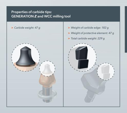
> WIRTGEN Compact Carbide (WCC) milling tools with an extremely robust carbide edge are particularly suitable for stabilising compact soils which contain large pieces of rock. This makes the WCC tools a useful alternative to conventional picks for these requirements.
