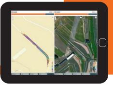
Live mode not only indicates geographical position in various map views, it also displays process data (e.g number of passes, asphalt temperature HMV value) for each point, machine and drum individually
