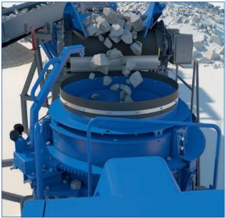
As soon as levels have dropped in the overfilled plants, the feed speeds are automatically raised again.
