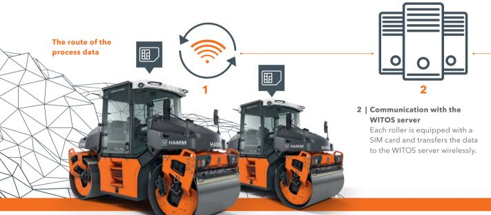
Random sampling and point measurements in the compaction process will soon be a thing of the past. The HCQ Navigator from HAMM is a highly effective alternative. The intelligent compaction measurement assistance system indicates compaction progress to roller operators, enabling them to produce homogeneously compacted surfaces.
