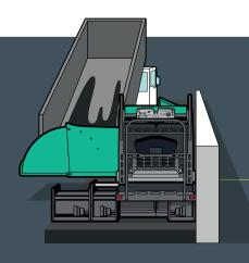
With the optional asymmetrical hopper (left), the paver can be supplied with material by lorry even if the feed vehicle is unable to dock centrally in front of the machine, as is the case when paving along walls or other boundaries.
