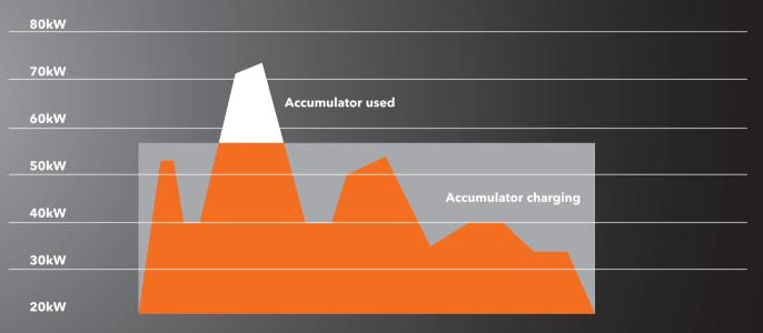
The distribution of labour in a power hybrid drive: the diesel engine delivers all the power required for most working situations. But sufficient power reserves (orange) remain, enabling the hydraulic accumulator to be filled for use when next required. Whenever the maximum load (white) is called for, the hydraulic system supplies additional power.
