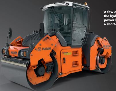
A few components with a big impact: the hydraulic accumulator on HAMM's power hybrid roller repeatedly supplies a short-term load of 20kW.
