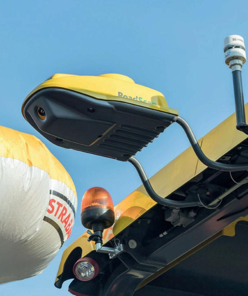
Documentation with practical benefits: RoadScan provides contractors with proof of paving quality and offers their paver operators a way to keep track of the temperature of the supplied mix - on the display of the paver operator's ErgoPlus 3 console.
