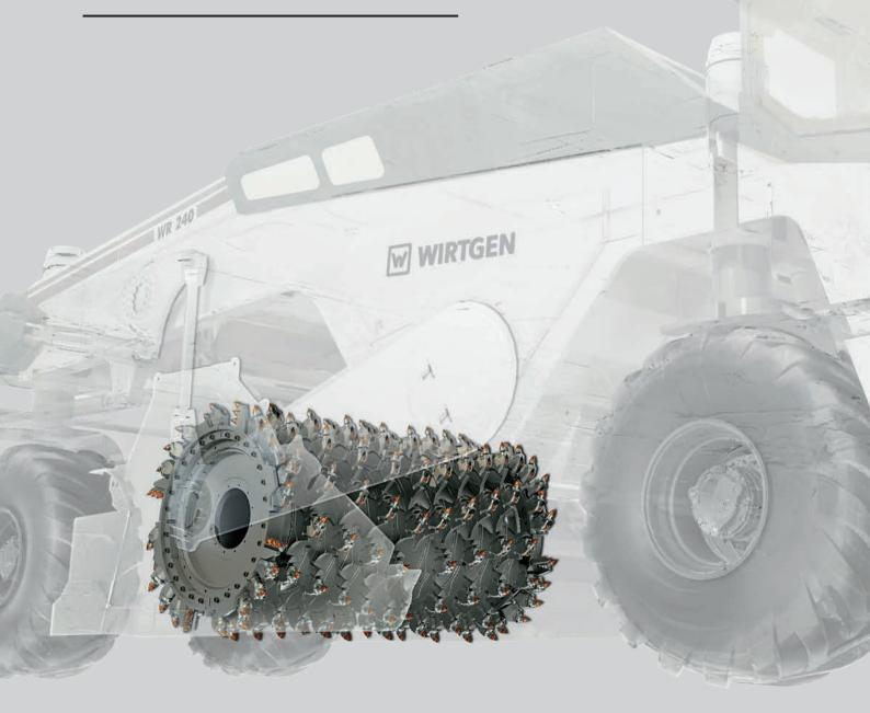
With its centrepiece, the DURAFORCE milling and mixing rotor, the WR series guarantees success in cold recycling and soil stabilization.
