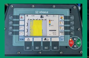
Unique precision: VÖGELE's temperature-measurement system sets standards.
