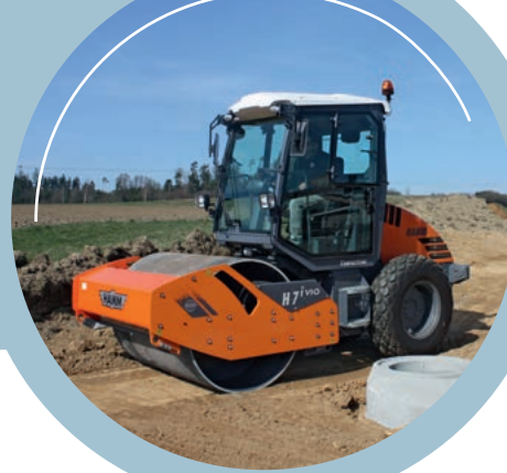
Compacting the roadbase around existing installations (manhole covers etc.) in a new housing development in Münchberg, Germany: the compact HAMM H 7i VIO compactor is in its element on jobs like this. Thanks to the VIO drum, this compactor can operate with either oscillation or vibration.
