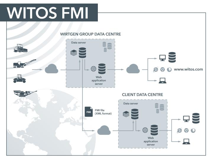
> The Fleet Management Interface (FMI) also allows you to import data from existing systems via a standardised server-2-server interface.
