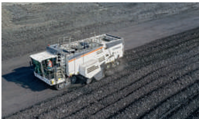
The Surface Miner 220 SM (i) 3.8 with a 3.8-m-cutting drum for the efficient extraction of soft rock and stone.
