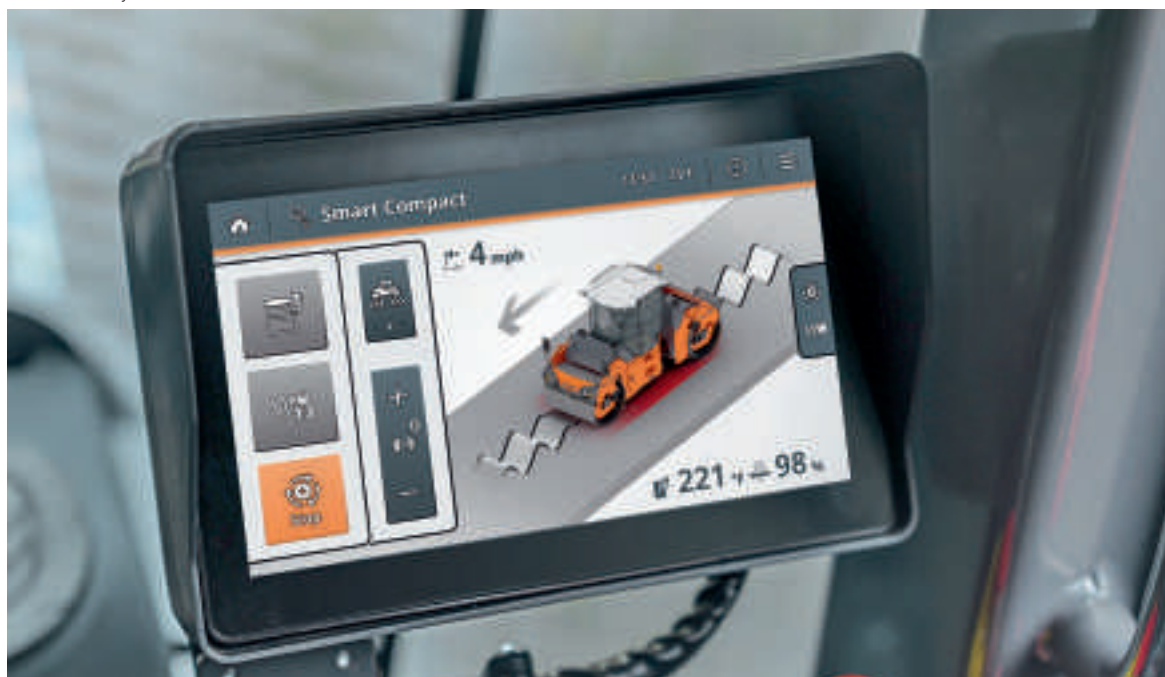
Smart Compact Pro for automated compaction in road construction on the basis of the real-time density.
