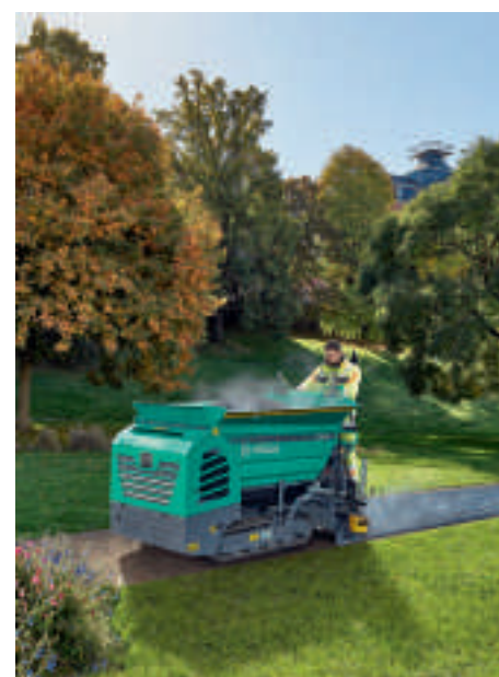
The smallest VÖGELE paver can accomplish paving widths as narrow as 0.25 m.
