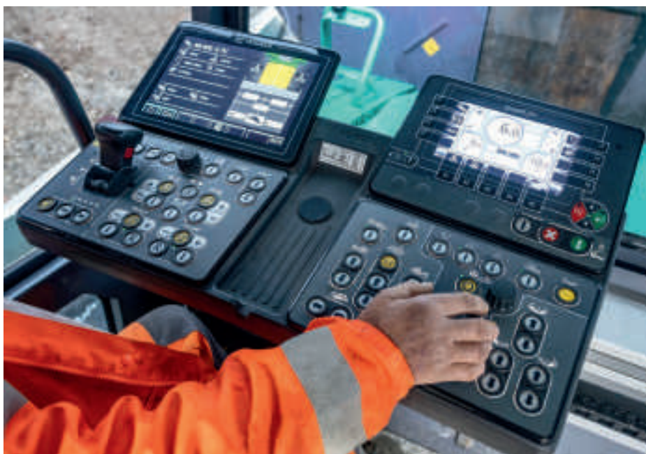
Focus on users: The ErgoPlus 5 operating concept is clearly laid out, ergonomic, and with the optional touch display, offers all prerequisites for digital road construction.
