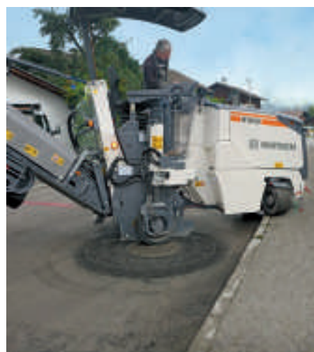
Milling around obstacles such as manhole covers with the highly maneuverable small milling machines.
