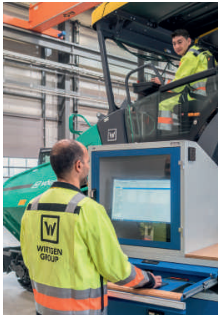
Helps with fast error diagnostics: the WIDIAG Service-Diagnostics System
