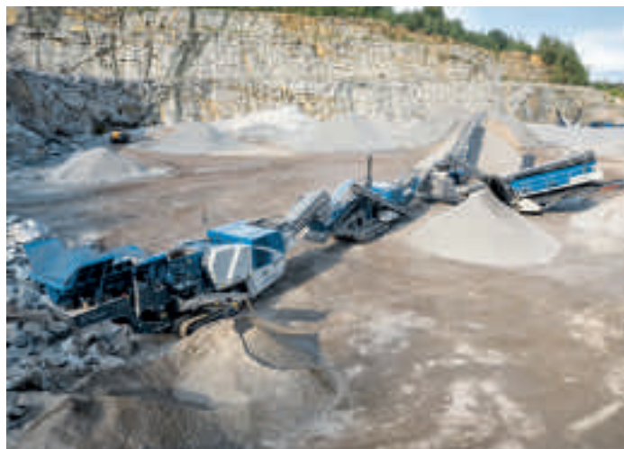
Optimum material processing through multi-stage crushing and screening processes.
