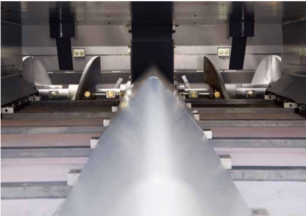
The conveyor can be reversed at the touch of a button. Return transport of the mix is automatically stopped. The conveyor can be switched to the no-load function just as quickly.
