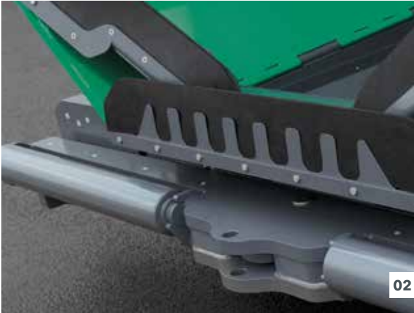
01 Independently operated hopper wings. 02 Large oscillating push-rollers can be set to 2 different positions for convenient and shock-free docking of feed vehicles even in curves.
