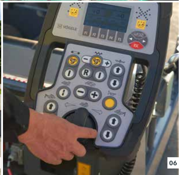
04 PaveDock Assistant communication system for optimum material feed 05 Large material hopper with a capacity of 28,660 lbs. (13 tonnes) 06 ErgoPlus 3 screed operator's console with SmartWheel for convenient screed width control
