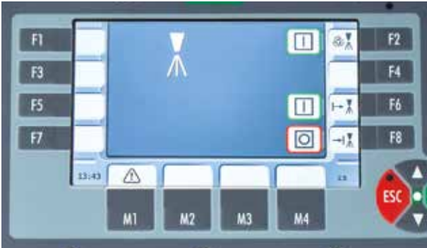
“Start of Job” and “End of Job” The convenience functions “Start of Job” (F6) and “End of Job” (F8) are provided so that spraying always starts and ends at exactly the required point and continues over full paving width.
