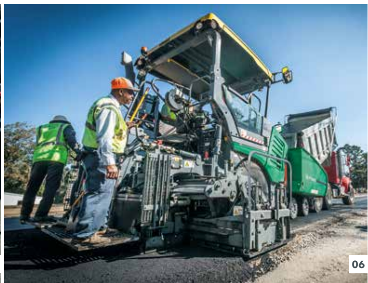
04 ErgoPlus 3 with numerous additional ergonomic and functional advantages. 05 Optimum feeding with mix thanks to the large material hopper. 06 The right screed for every application. The paver can be combined with the VF 500 and VR 500 Extending Screeds.
