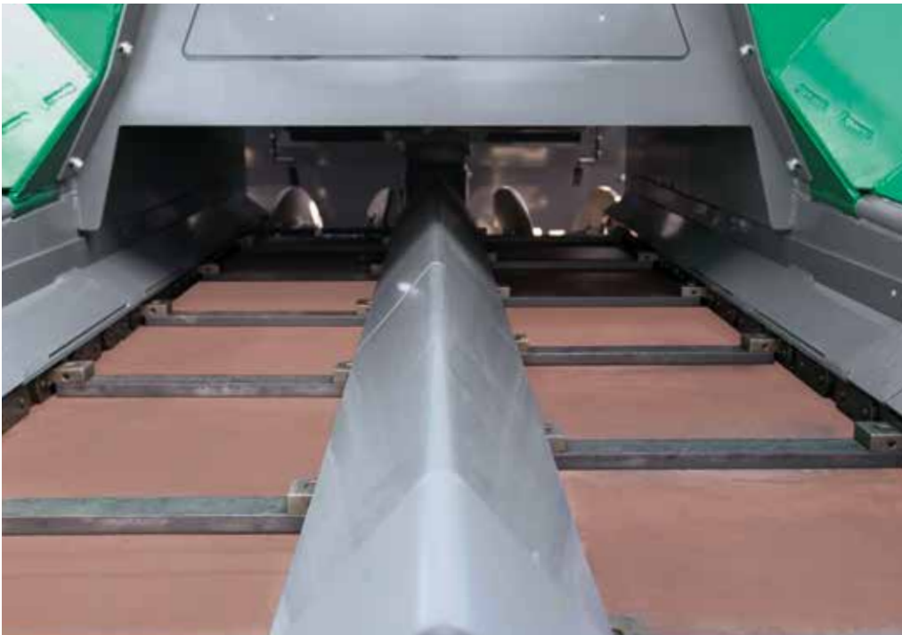
Narrow conveyor guard in the material hopper guarantees uniform material flow.
