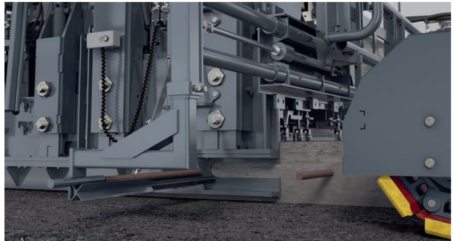
Separate side tie bar inserter.
