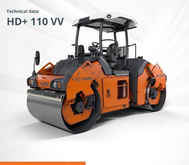
Tandem rollers Series HD+ Tandem roller with two vibrating roller dru H258
