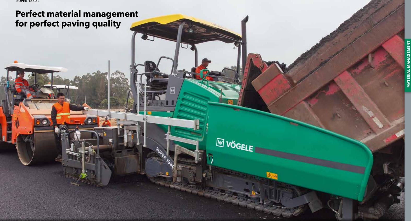
A continuous flow of mix is key to ensuring uninterrupted and high-quality paving. That is why we attach such importance to professional material management when designing our pavers. This is also essential if this multifunctional paver is used for roadbase applications.
