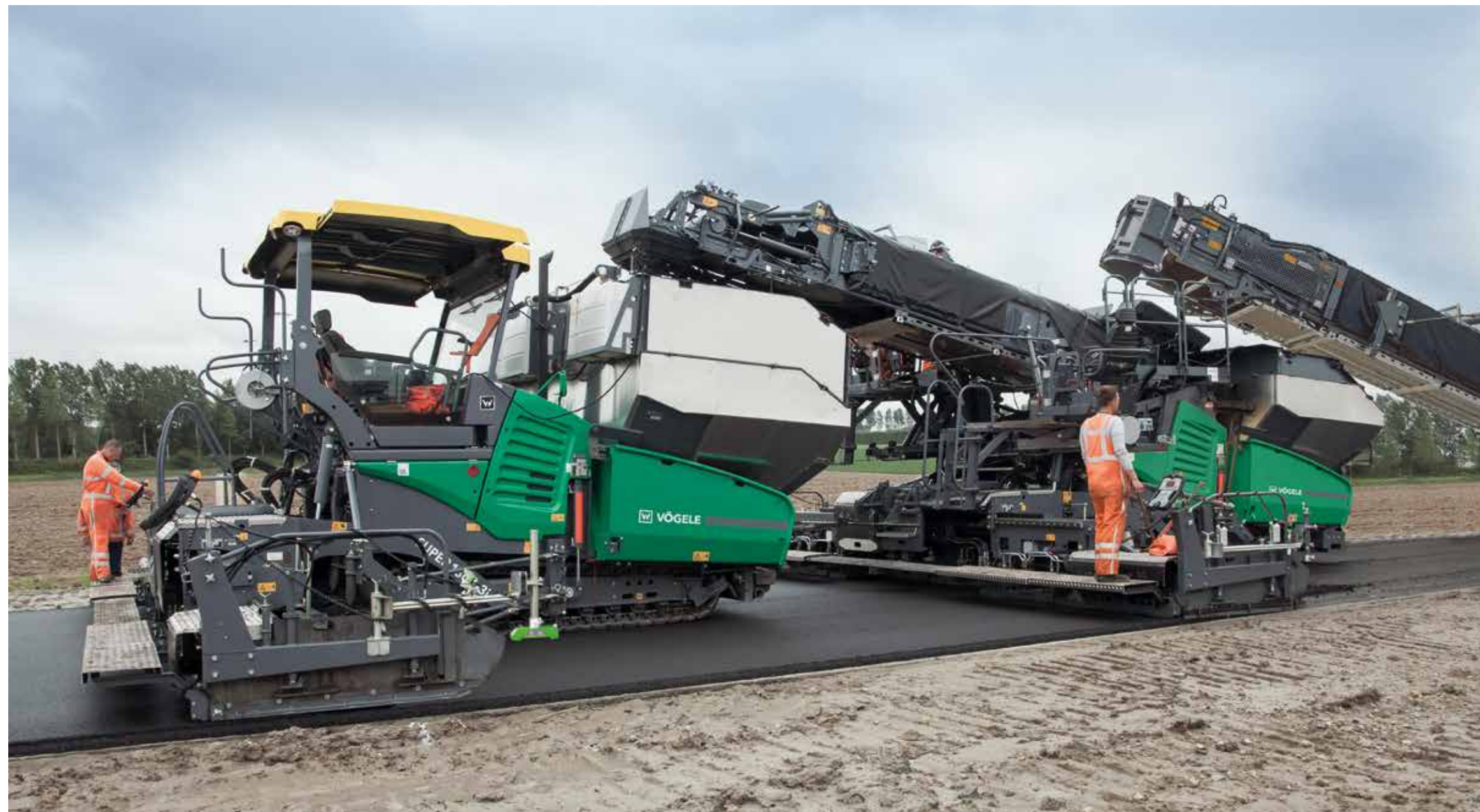
Two height-adjustable operator's stands give the operator an optimum view of the entire workflow on the job site.
