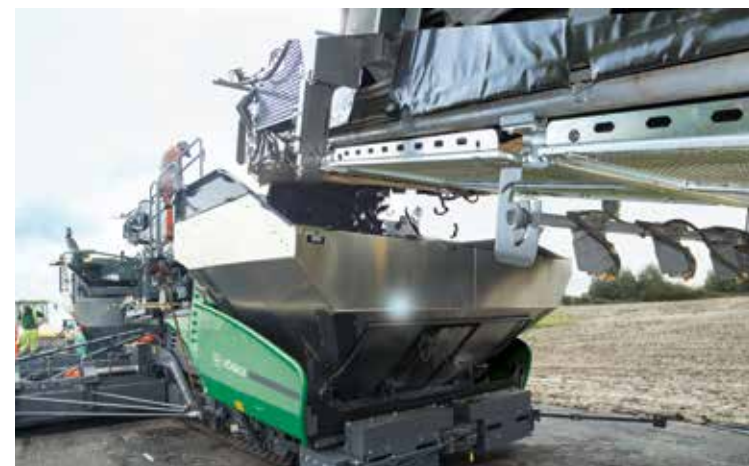
The conveyor of the transfer module is heated in order to prevent mix from sticking.
