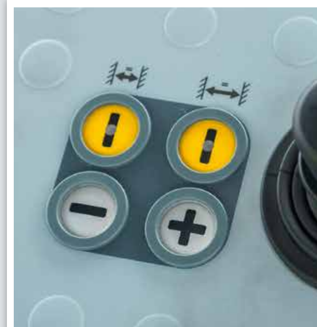
For automatic distance control the operator can select between two different distances.
