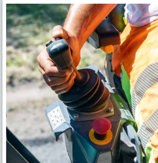
The pivoting conveyor is controlled via a joystick in the armrest of the operator's seat.
