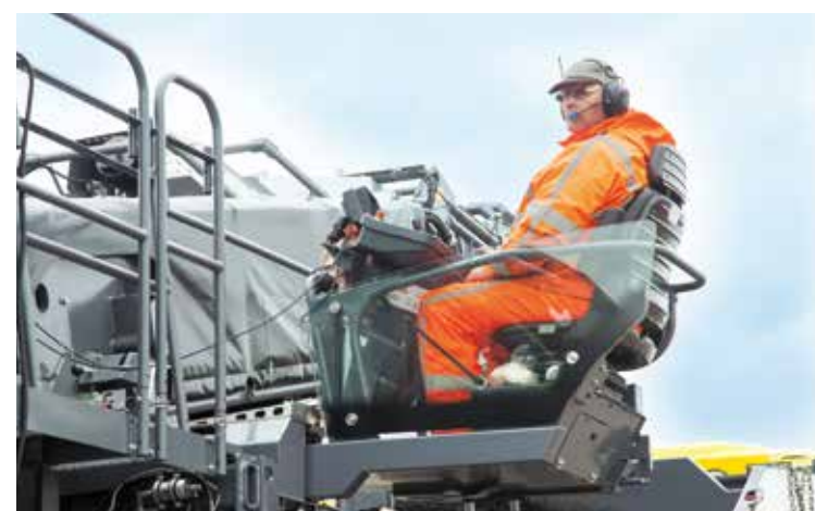
Two height-adjustable operator's stands give the operator an optimum view of the entire workflow on the job site.
