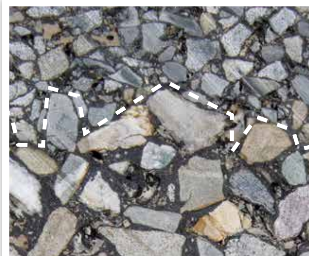
Excellent bond and interlocking of binder and surface courses
