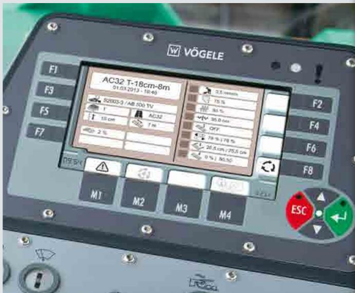
The automatic Paving Programs function allows the operating personnel to store their own paving programs. All key parameters for paving a specific layer (example: base course of asphaltic concrete, 18cm thick) can thus be saved.
