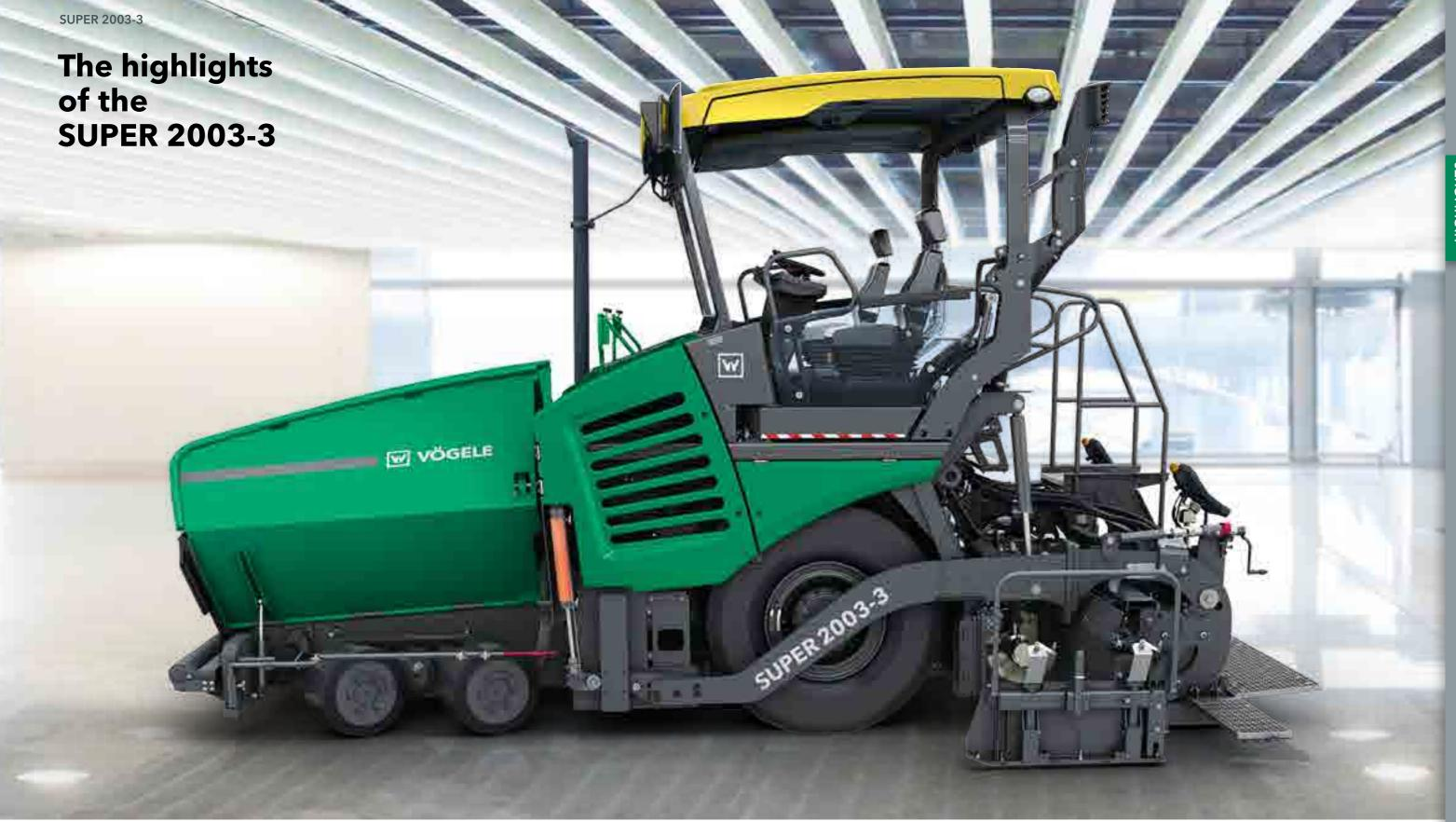
Wheeled Highway Class paver with a large range of applications and pave widths up to 7.75m **Powerful and economical drive concept** with VÖGELE
