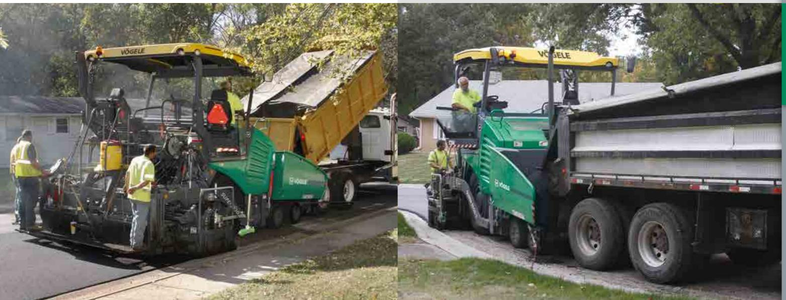
The hydraulically operated hopper front prevents material spills during lorry exchanges. It directs the material inside the hopper directly onto the conveyors, so no hand work is required. All of the mix is properly conveyed to the screed.
