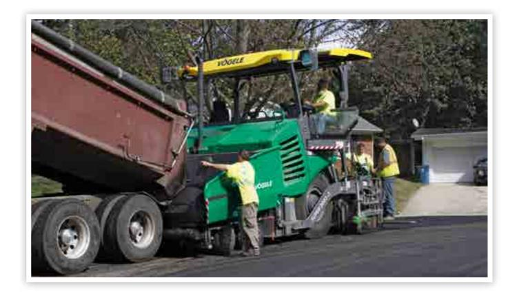
With the SUPER 2003-3 VÖGELE have now developed an entirely new paver which has been designed for markets where high pave speeds are required. The wheeled SUPER 2003-3 is designed primarily for use in highway construction and large-scale commercial applications, which are all about power and productivity. With a powerful, 6-cylinder Cummins engine rated at 179kW and high-output hydraulic drives, it is fully equipped for these jobs.
