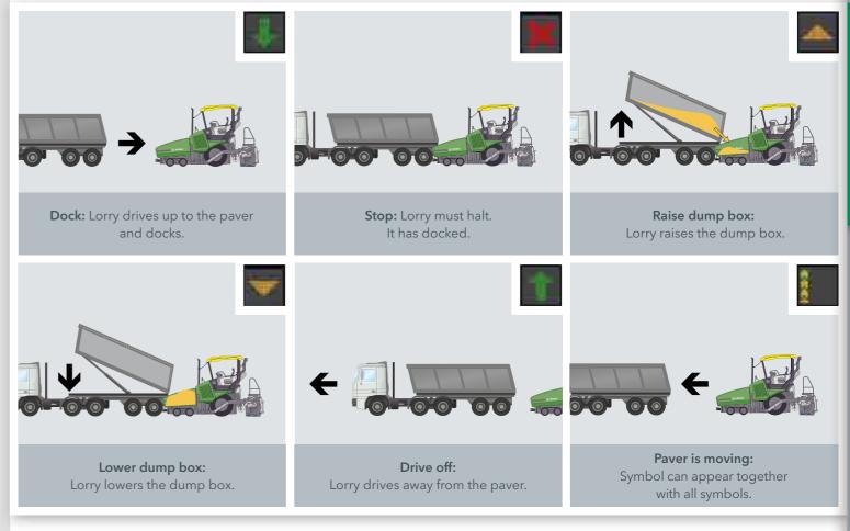
**PaveDock Assistant** is the communication system between the paver operator and the driver of the feed vehicle. It allows particularly fast and reliable transfer of mix to the paver. Signal lights on the paver and the associated controls on the paver operator's ErgoPlus 3 console are key components.
