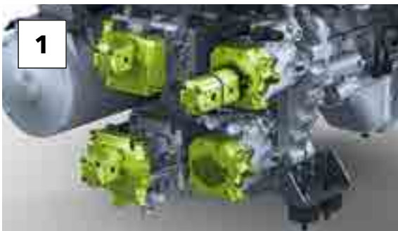
Splitter gearbox with ability to disengage hydraulic pumps
