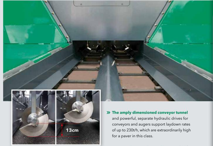
The height of the augers is infinitely variable by 13cm for uniform spreading of mix across the entire pave width.
