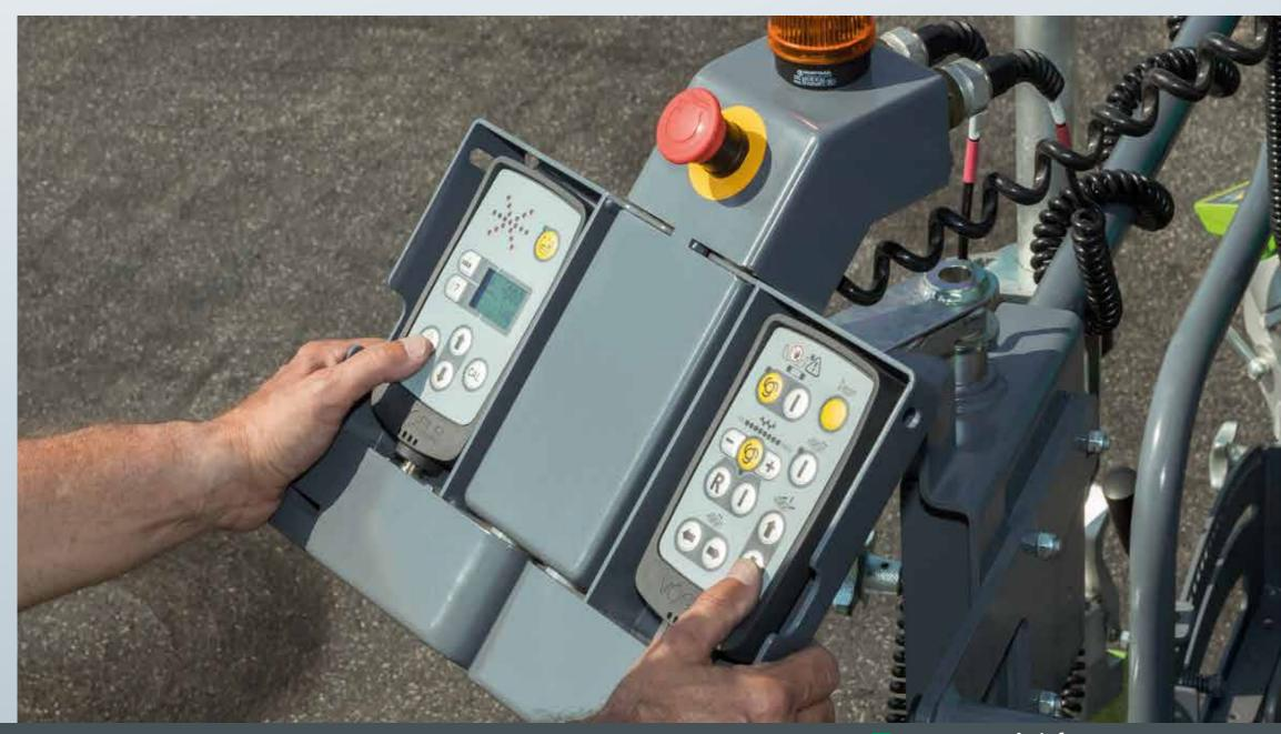
**The remote control units** cover all the functions required for high-precision grade and slope control. Clear symbols support intuitive machine operation.
