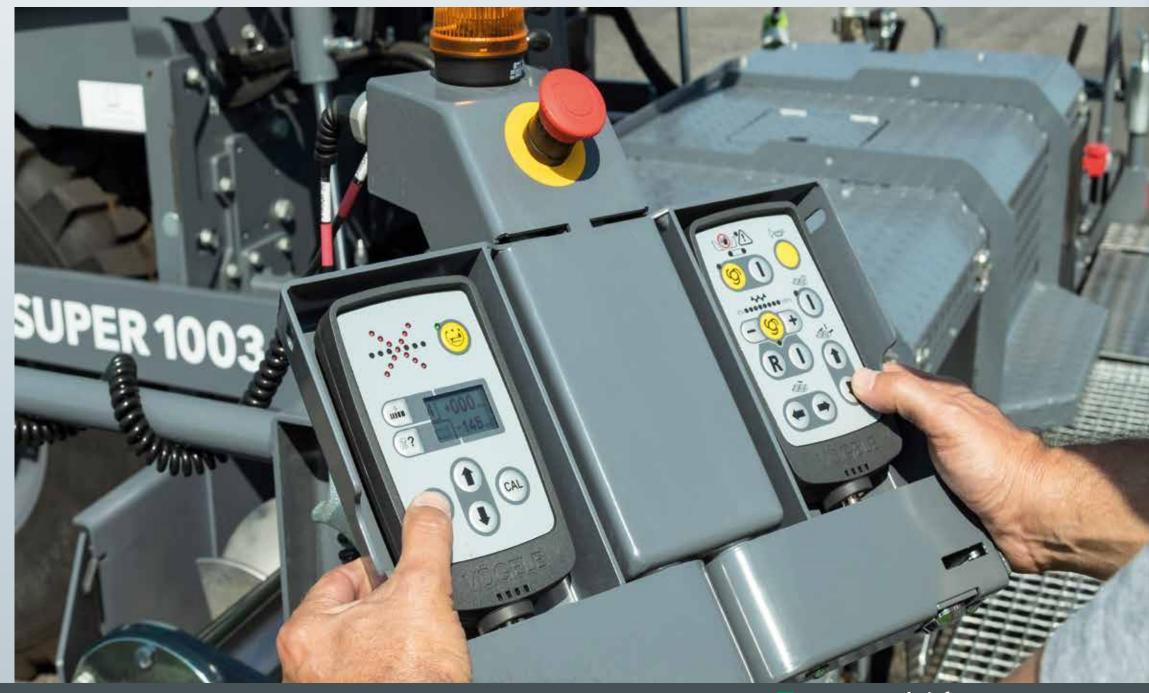
All the main paving functions can be controlled using the two handy remote control units for the screed. Simple, language-neutral symbols allow the machine to be operated intuitively.
