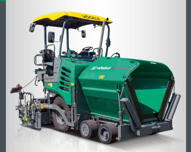
Maximum pave width 3.9m Maximum laydown rate 230 tonnes/h Transport width 1.85m
