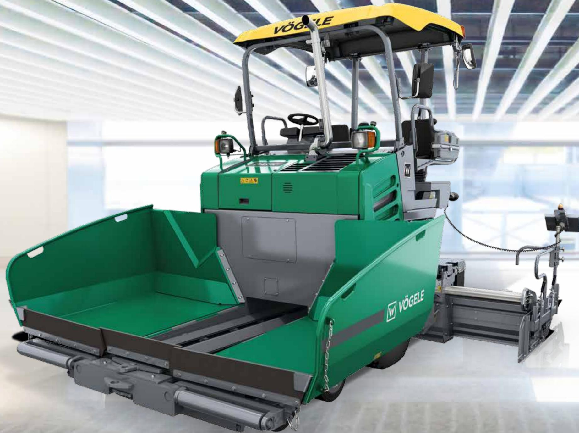
**Wheeled Compact Class paver** with a wide range of applications and pave widths up to 3.9m
