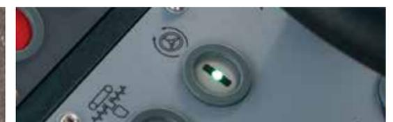
**Highly manoeuvrable** thanks to Pivot Steer. With Pivot Steer activated, the rear inside wheel is automatically slowed down hydraulically. This minimizes the outside turning radius to no more than 3.8m for positioning manoeuvres and paving. The function can be activated in "Pave" and "Positioning" modes, greatly increasing the manoeuvrability of the machine on confined job sites.
