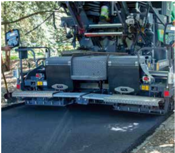
AB 340 built up with 25 cm bolt-on extensions
