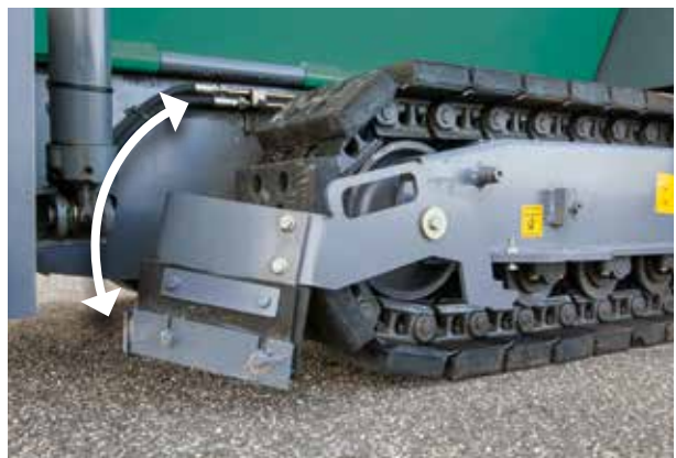
RAISE/LOWER DEFLECTORS IN FRONT OF THE CRAWLER TRACKS
