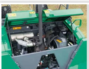
**Powerful** diesel engine develops 116kW at just 2,000rpm.
