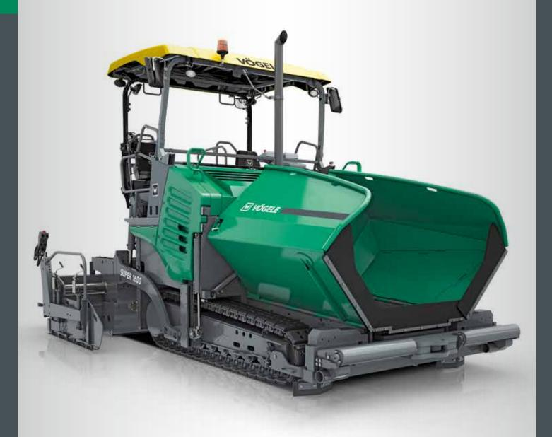
Maximum pave width 6.3m Maximum laydown rate 600 tonnes/h Transport width 2.55m
