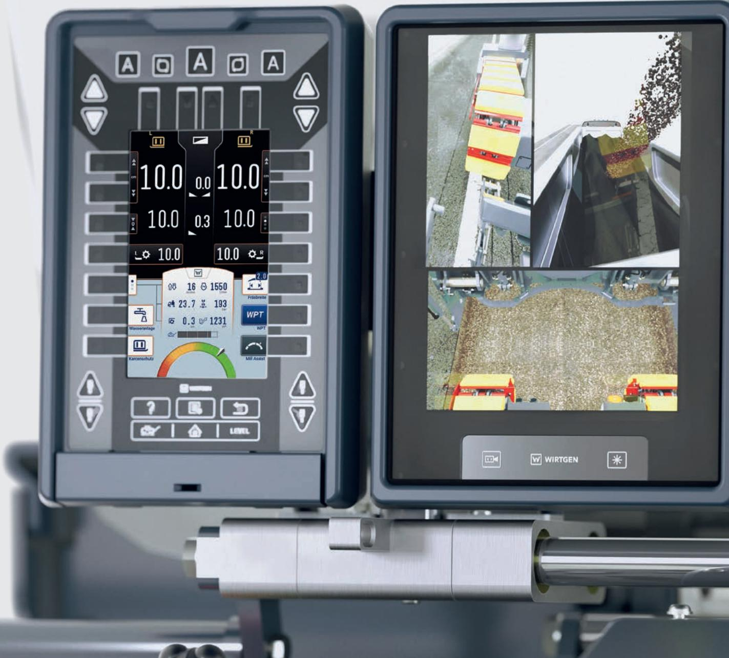
**1 |** 10" control panel with split screen feature for the simultaneous display of multiple camera images.
