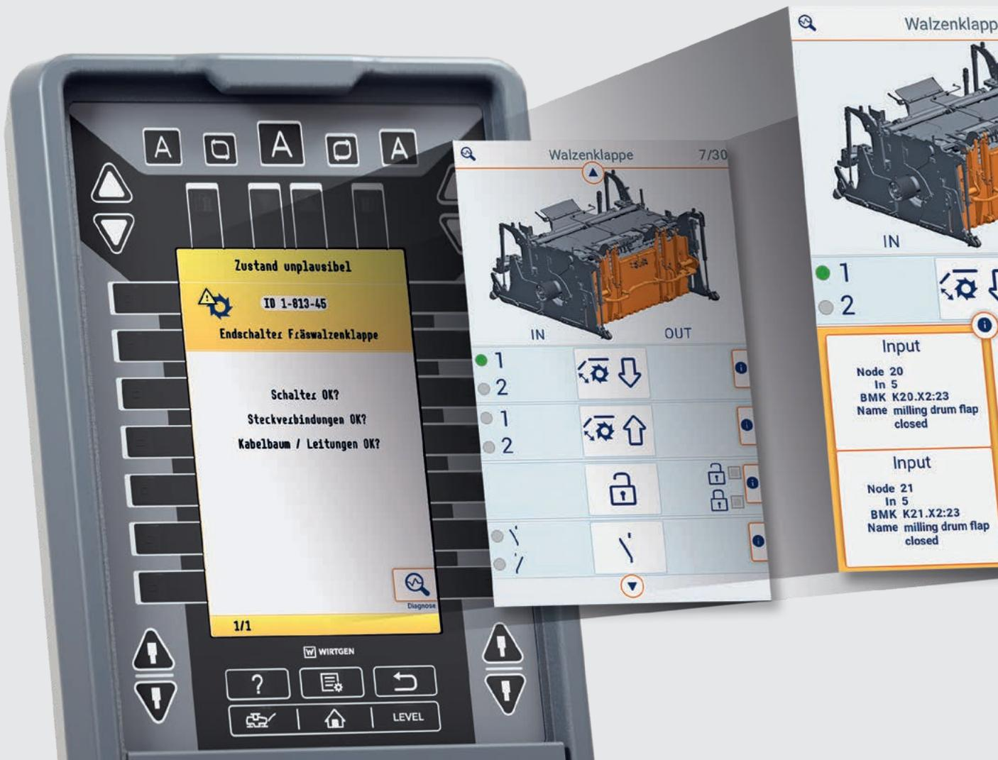
**1 |** Direct forwarding of the image from the error message to the diagnostic system including clear location of the fault.
