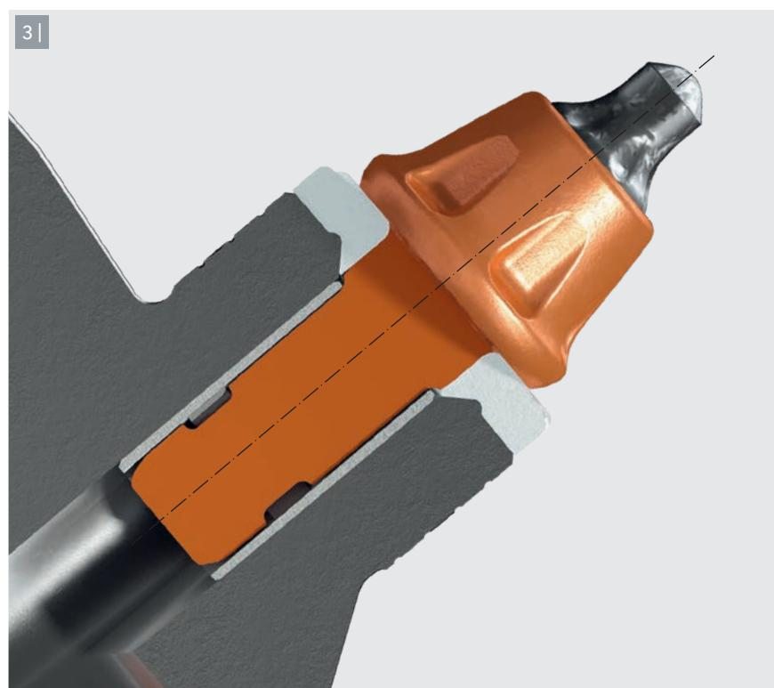
**3 |** In combination with the new pick, the centring embossment on the new toolholder optimizes rotation to reduce wear and tear.
