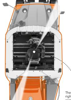
The driver sits on the left or right of the platform while compacting, looking past the engine cover or water tank, respectively. This means that he has the construction site in view at all times.
