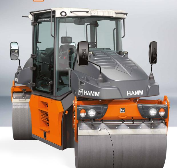
The water volume can be finely adjusted in five stages directly from the driver's seat. It is automatically regulated as a function of the speed.
