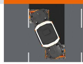
The large track offset makes it possible to almost double the working width in relation to the drum width.
