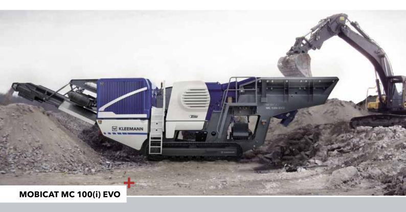
The smallest mobile jaw crusher of the EVO line impresses with its compactness and reliability. Can be used for the most varied of materials, the plant offers wide-ranging possibilities for both demolition companies and contract crushers. Thanks to diesel direct-drive, the MC 100(i) EVO has a lower fuel consumption.
