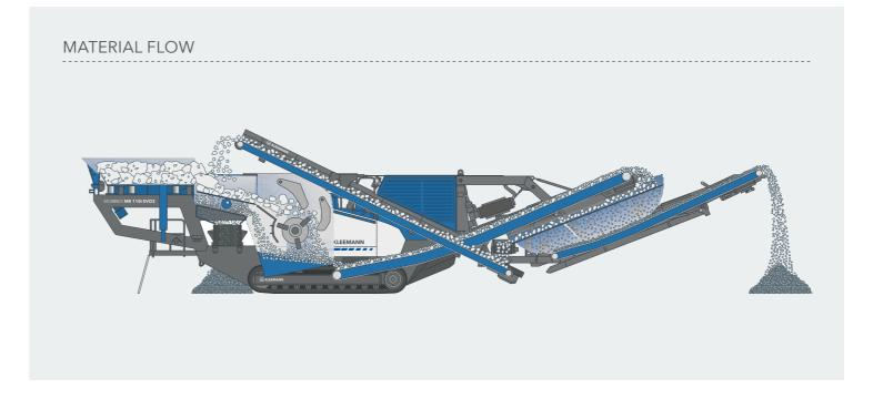
The MOBIREX MR 110(i) EVO2 stands out with its optimal material flow concept: The system widths are extended over the entire plant in the direction of material flow. This means that the material flow is not restricted and material bridging can be effectively avoided. The Continuous Feed System makes the operator's work easier,
