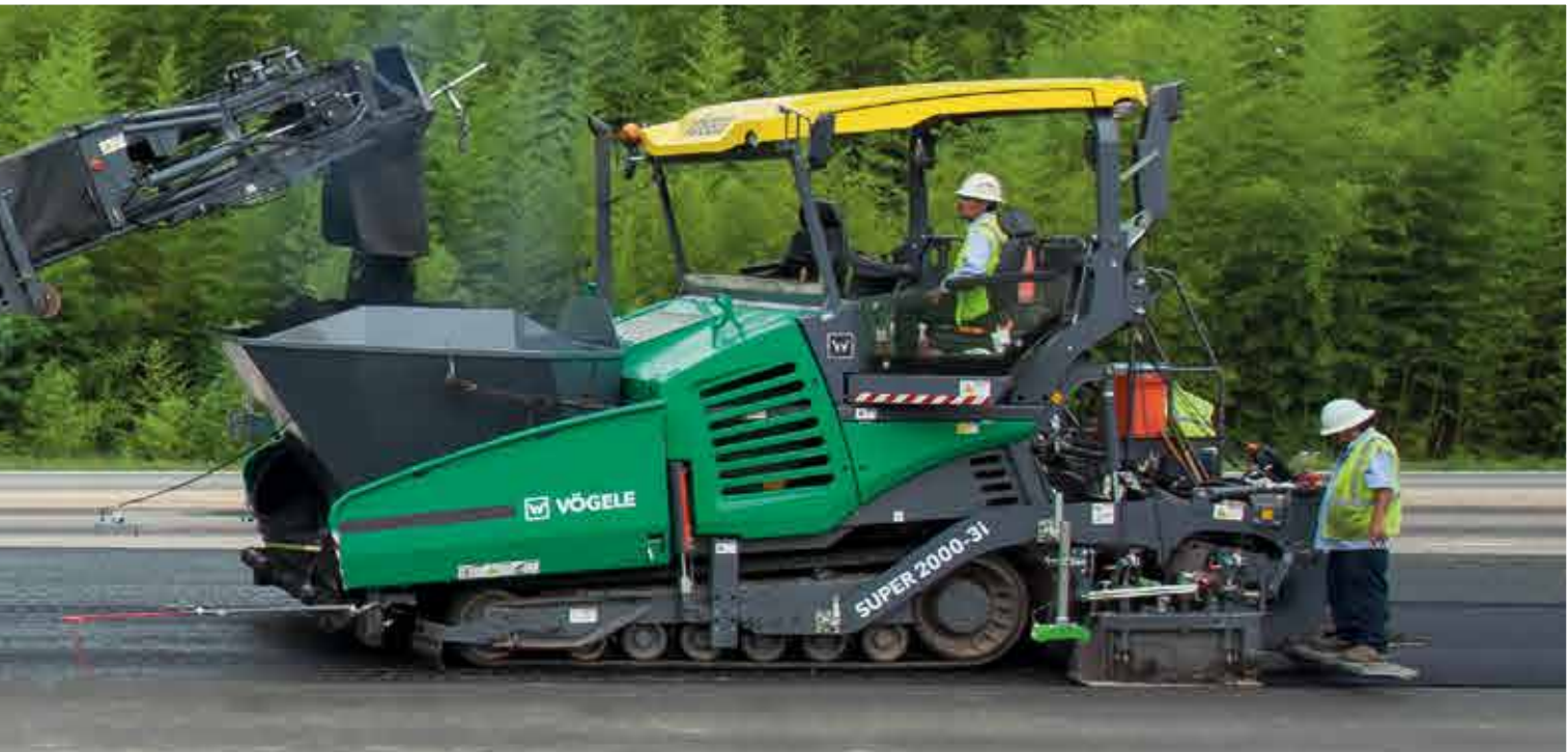
The power unit of the SUPER 2000-3i with diesel oxidation catalyst (DOC) and selective catalytic reduction (SCR) for exhaust gas after-treatment complies with the strict requirements of European exhaust emissions standard Stage 4 and US EPA standard Tier 4f.
