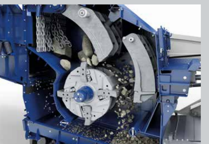
Crusher unit with optimised inlet geometry
