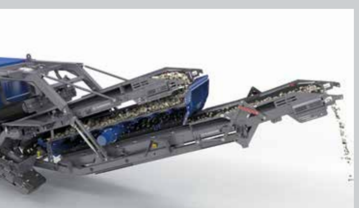
Vibrating screen with extra large screening surface
