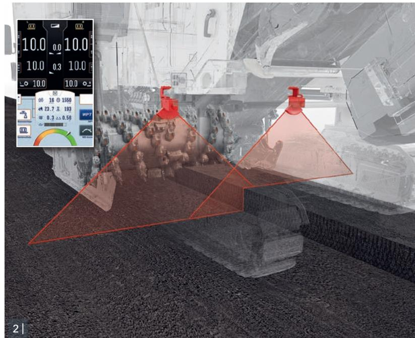
**1 |** The operator is provided with continuous information on the current machine and job parameters - at the end of work, the data are transmitted to the machine user.
