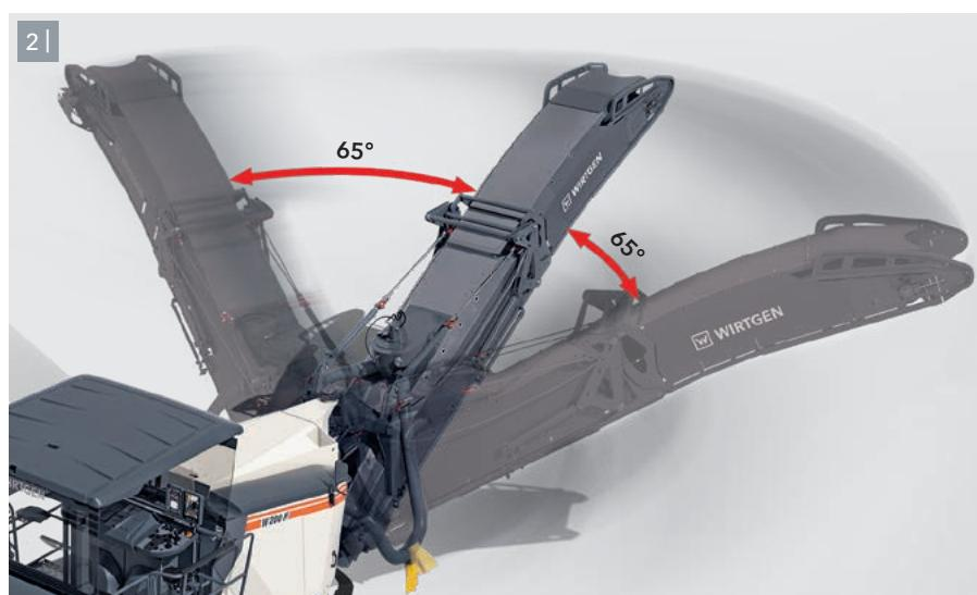
**1 |** Increased scraper lift for a wider range of milling applications and reduced wear.
