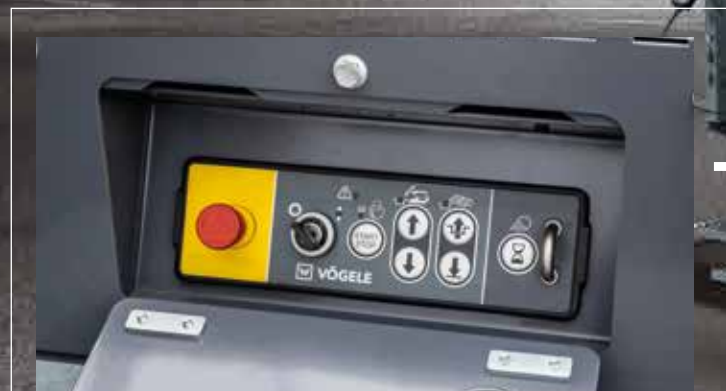
Paver Access Control Unit for convenient and safe access to the paver.
