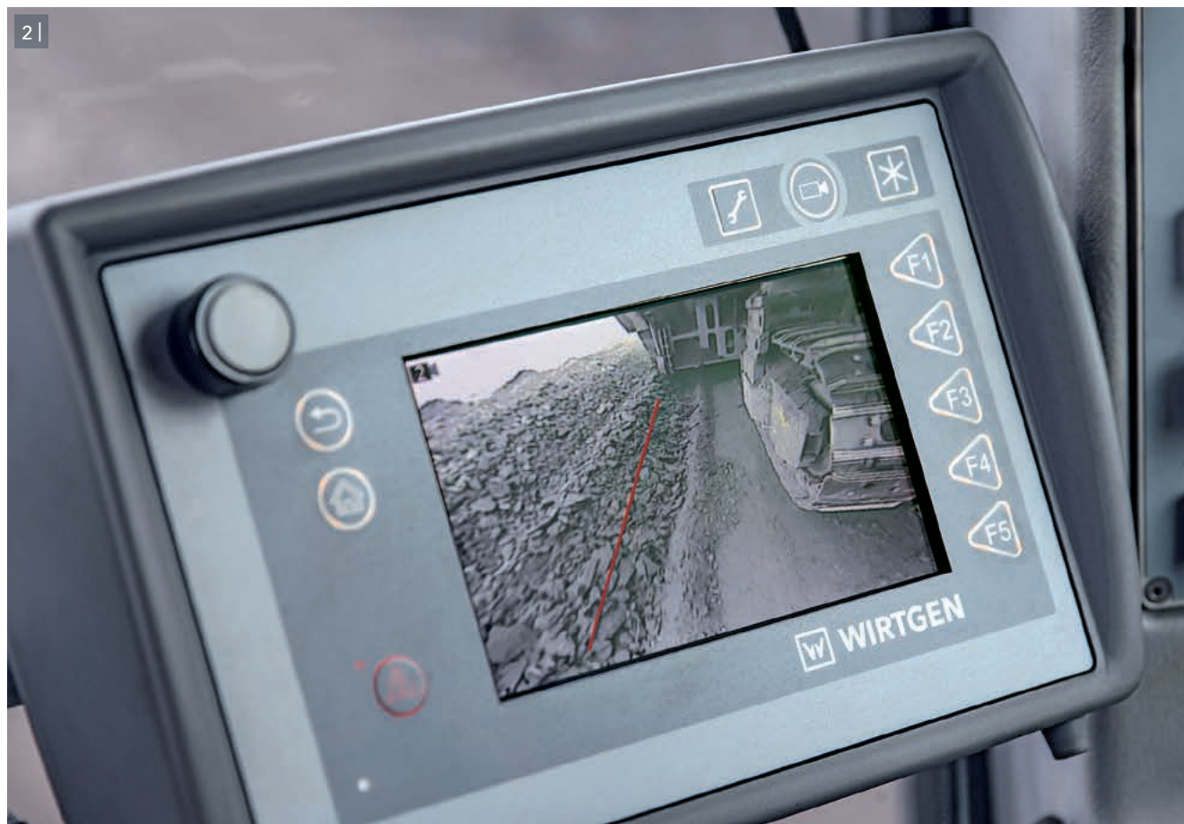
2 | Quick manoeuvring using the reversing camera improves the overall productivity of the machine.
