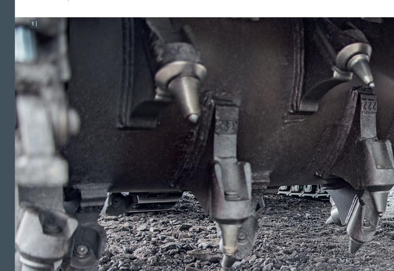
1 The picks are arranged in a specific pattern tailored to the windrowing method.
