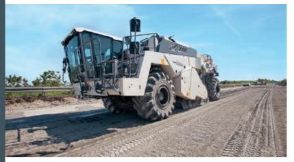
The WR 240 impresses by paving the base true to line and level as the automatic cross slope control prevents any displacement of material on the previously produced subgrade level. The mixing concept with perfectly matched rotor and rotor housing produces mixes of superior quality in a short period of time, enabling the WR 240 to stabilize at high advance rates.
