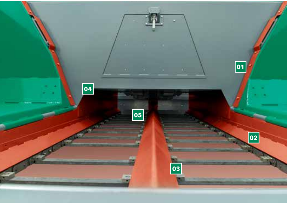
Components particularly protected by the Heavy-Duty kit (shown in red): 01 Scraper for the hopper sides 02 Lateral guards of the conveyor chains 03 Central guard of the conveyor chains 04 Conveyor tunnel 05 Centre auger bearing box
