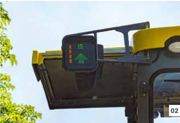
01 Choice of engine speed ranges 02 PaveDock Assistant (option)
