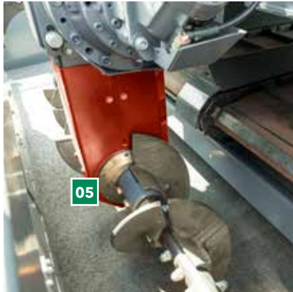
Components particularly protected by the Heavy-Duty kit (shown in red): 01 Scraper for the hopper sides 02 Lateral guards of the conveyor chains 03 Central guard of the conveyor chains 04 Conveyor tunnel 05 Centre auger bearing box
