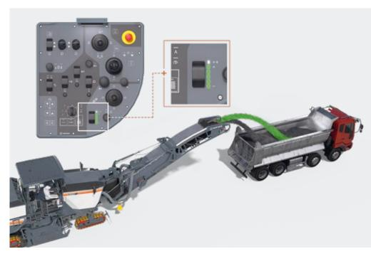
Booster function for a brief increase of the speed and conveying capacity of the discharge conveyor by 20%.
