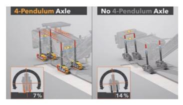
Four-way pendulum axle
