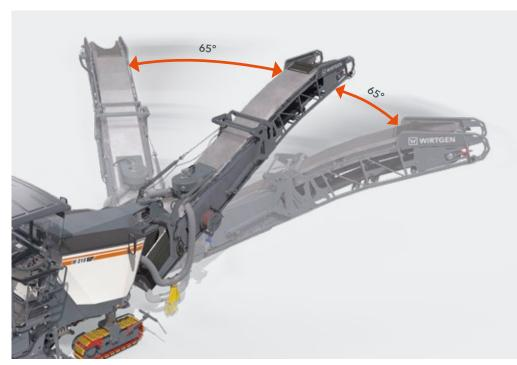
The discharge conveyor has a large swing range.
