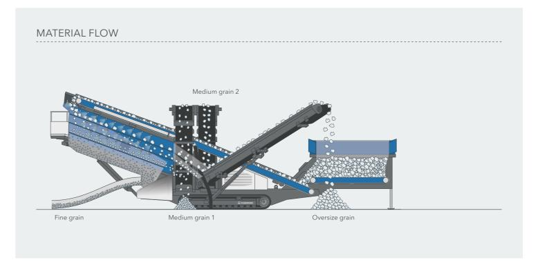
Thanks to compact transport dimensions, short set-up times and a large selection of screen media, the MSC EVO classifying screening plants can be used flexibly. In order to process large quantities efficiently, the material flow is designed optimally: starting with the feed hopper, which is widened in the material flow direction, to the wide feeding conveyor through to the generously dimensioned
