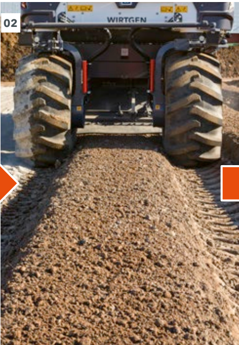
01 - 03 Stabilization transforms sub-bases with insufficient bearing capacity into soil that is suitable for paving and compaction.
