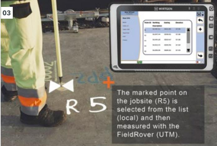
The marked point on the jobsite (R5) is selected from the list (local) and then measured with the FieldRover (UTM).
